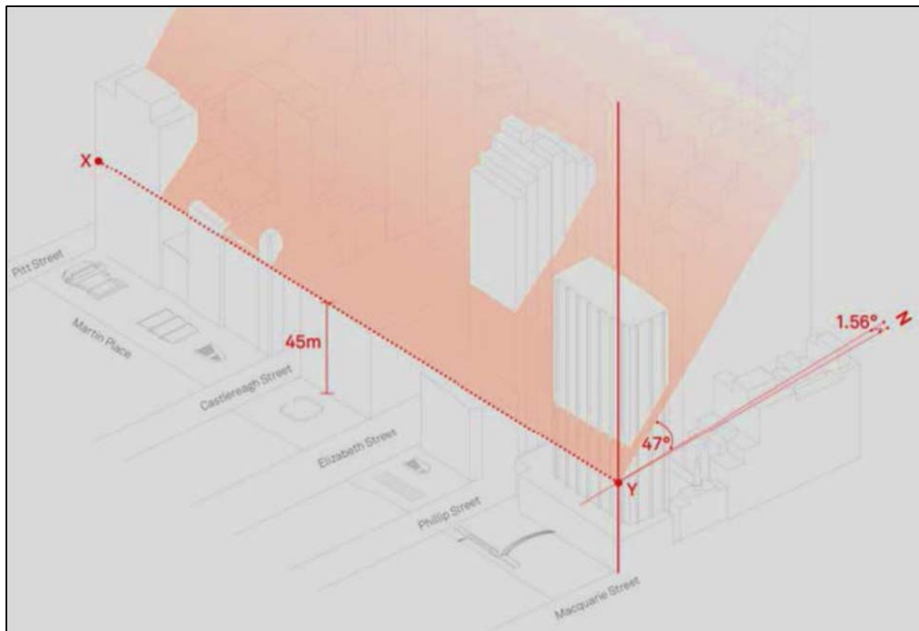
Figure 6: Derivation of the Martin Place 5B sun access plane, with 60 Martin Place projecting through in the foreground.
