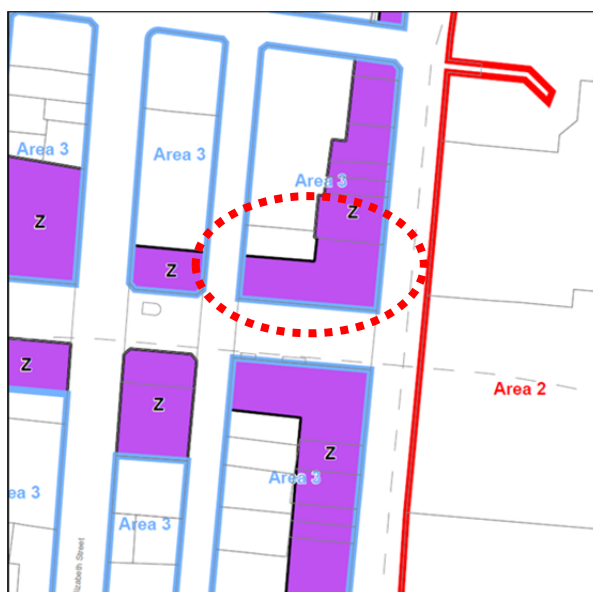
Figure 4 - Extract from Sydney LEP 2012 Height of Buildings map, with the site highlighted by the red dotted oval. Dark purple shaded areas have a height limit of 55m. White areas are subject to sun access planes.
