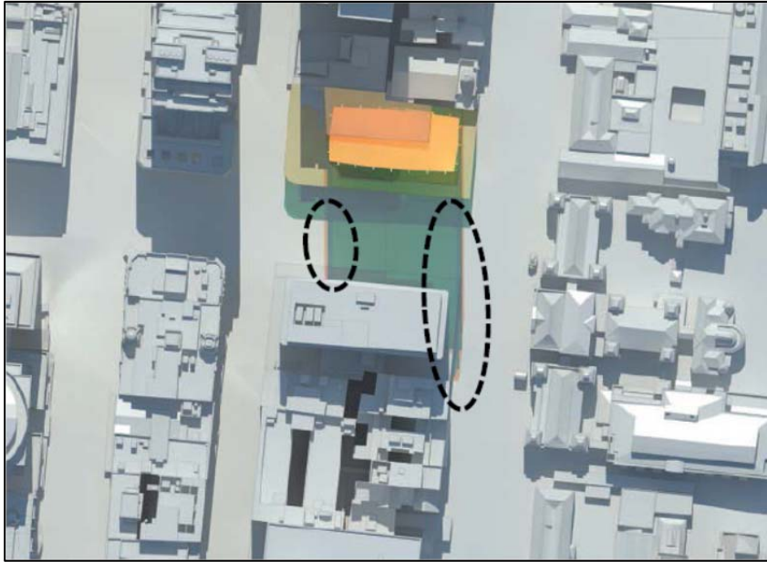
Figure 14: The additional shadow at 1pm on 21 March is highlighted, as the narrow orange colour on the margins of the existing overshadowed area, within the dashed black oval. It falls partly on the ground plane of Martin Place, and partly on Macquarie Street.
